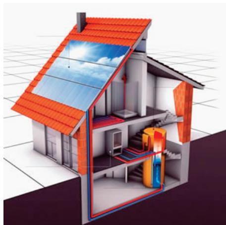
Figure 12: Diagram of a solar house (source: <http://www.pink.co.at/sonnenhaus.htm>)
