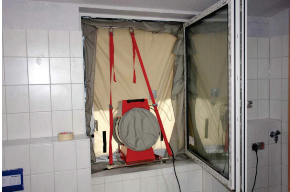
Figure 22: blower door test: in this case the device was built into a window because the front door was very likely to leak (source: Schulze Darup)
